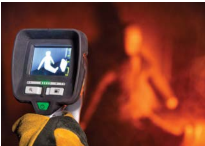
FIGURE 2: IMAGE OF THE "SMARTDUMMY THERMAL" ON A THERMAL IMAGING CAMERA
