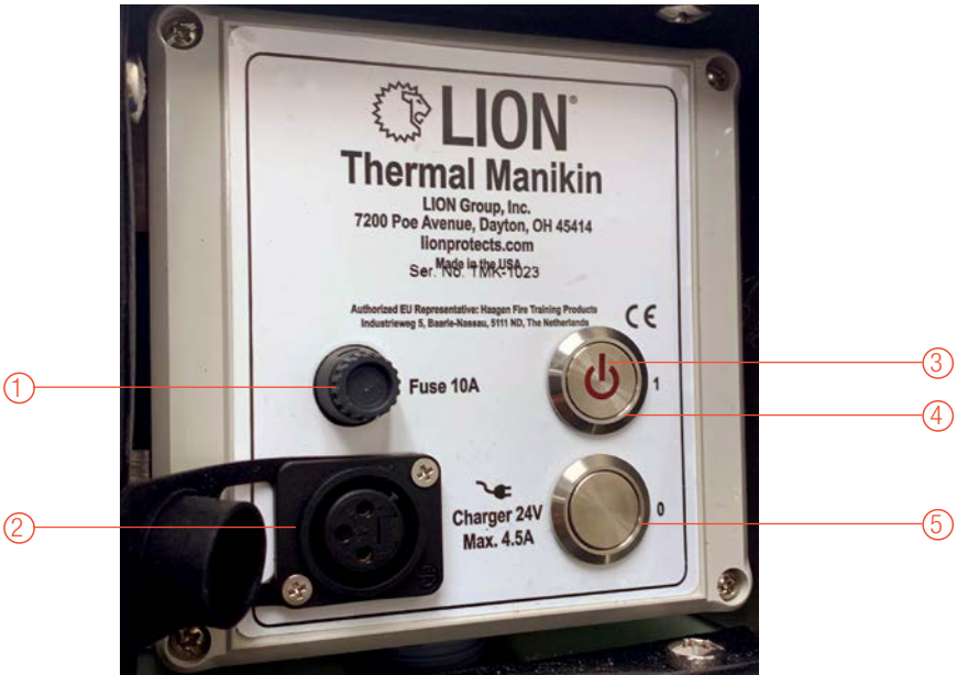
FIGURE 4: OPERATING PANEL “THERMAL MANIKIN”
